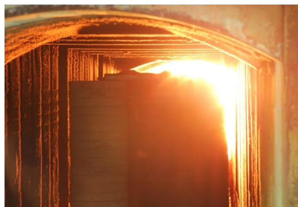
The continuous kiln maintains a temperature of approx. 1,460°C
